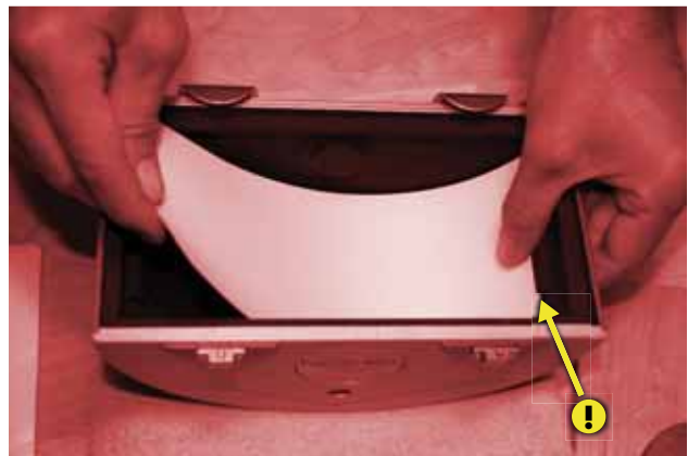
◄ Cross section view of camera showing proper position of paper/film. Notice how the photo material rests on top of the small strips beside the retaining strips.
